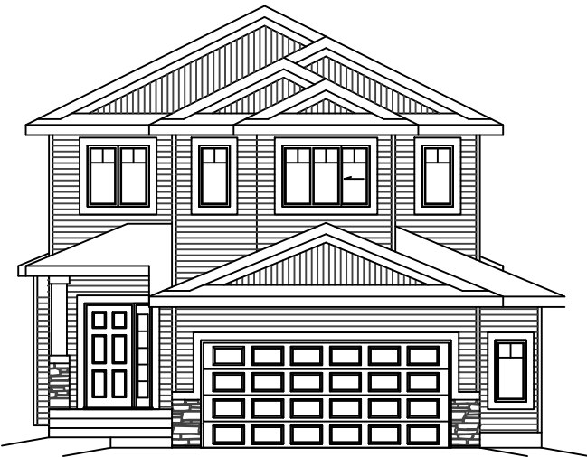
ELEVATION A- STANDARD 4'-0" GARAGE OFFSET 32' BUILDING POCKET
